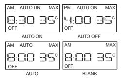
The booking timing mode setting can be circulated as above sequence and the yellow timing pilot light will be on during the heater operating in auto mode.
